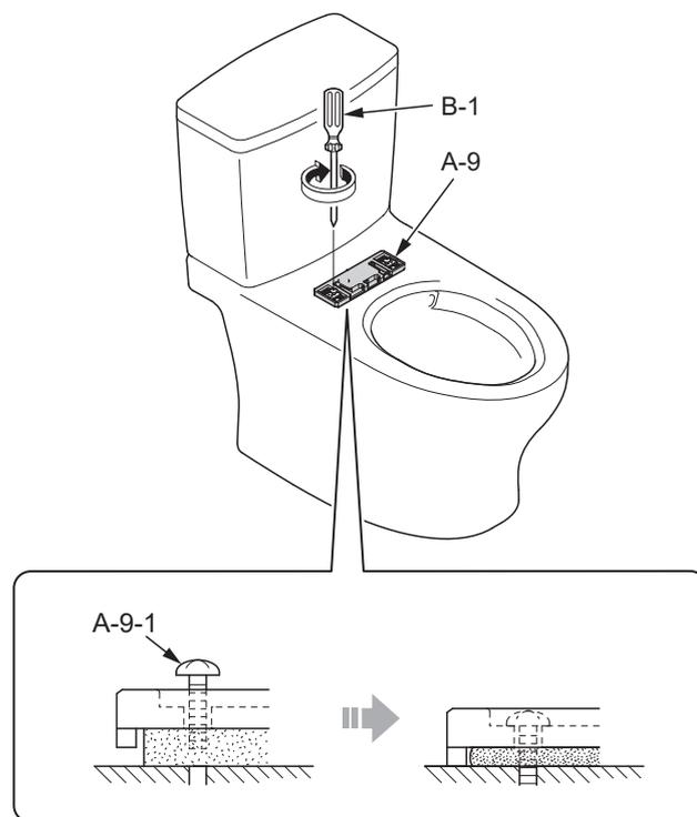
Failure to tighten screw A-9-1 completely will cause moving sideways of C-1.
