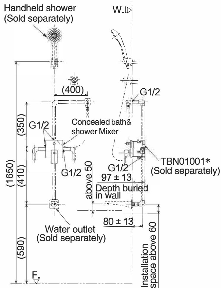
Note: The unit of size in the figure is mm
